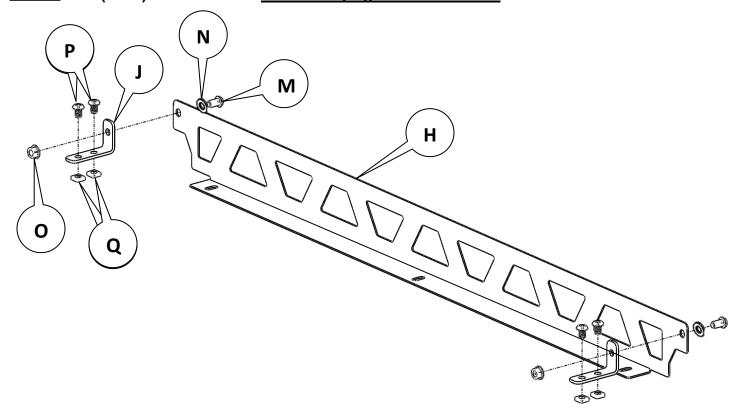
Slide the preassembled fences into the hex rails with the bends of the fences facing each other. The lower picture below is a side view of about where the fences and hex
