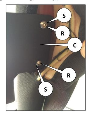
This step is for JL only, if you have a JK skip to step 5. Remove the plastic cover using the screwdriver on the driver side in the cargo area shown below to find the threaded holes.
