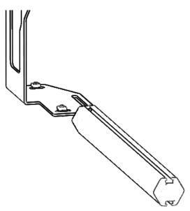
This Step is Optional. If you want tie downs, slide the tie down (L) onto the top side of the hex rails.
