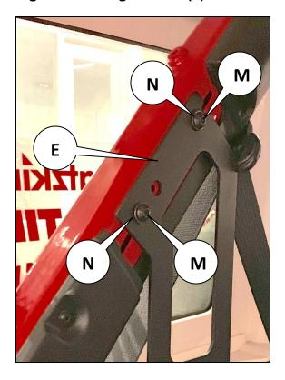
This step is for DZ 4470JP Steel Rack (A) only, if you have a DZ 4471JP Bolt Together Rack skip to step 6. Place steel rack onto brackets and use bolts (M), washers (N), and nuts (O), to install rack to brackets. Center the rack and tighten all hardware. Discard any extra hardware.
