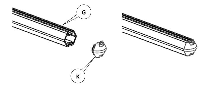
Slide the hex rails into the nuts from step 6.
